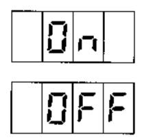
The buzzer should sound each time ON is displayed.
