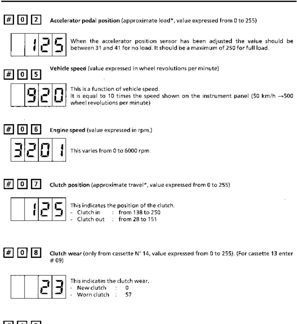
Accelerator pedal position (calculated load \*, value expressed from 0 to 255).
