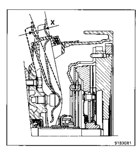
Reposition the pump assembly. It is supplied full of fluid.
